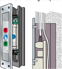
SLIM-DUALUX No-touch stop and go display type 5 for recessed assembly using flange and wall box.
