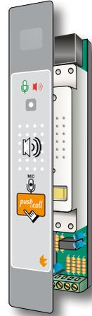
The talk-listen unit is the device that, when matched to another identical unit, in tandem and/or in multiples (with special Voxtronix centralisation module), allows voice intercommunication between different remote stations. The "Push&Call" button activates the start of the conversation in "alternated listen and answer mode". The two-colour LED (red/green) signals the current "Listen/Talk" status.
